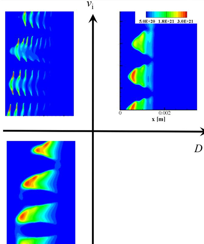
Observed (top) and computed (bottom) millimeter-wave discharge.
