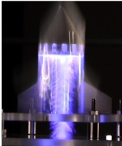
Atmospheric Millimeter-wave Discharge in a Rocket.
