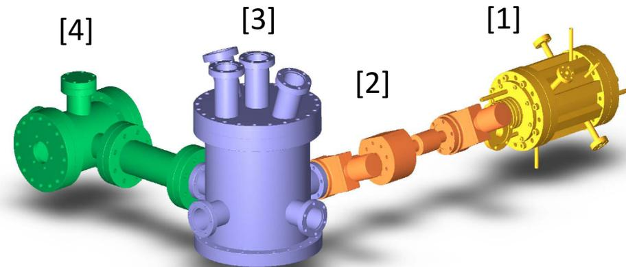
***Scheme of the experiment: [1] plasma source and Einzel extraction lenses, [2] neutralization by Cs vapor oven, [3] test chamber and Argon discharge, [4] UV spectrometer for Lyman- $\alpha$  light collection***
