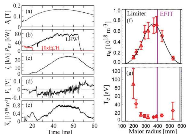
Figure 2. Waveforms of (a)  $B_t$ , (b) net RF (LH and EC) powers PRF, (c)  $I_p$ , (d) loop voltage  $V_L$ , (e) line-average density  $\bar{n}_e$ , (f) and (g) electron density and temperature profiles measured by Thomson scattering at 55 ms.
