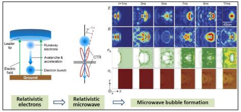
BL formation: Lightning first produces an intense electron beam, and then strong microwave is emitted when the electrons strike the ground. Microwave bubble is formed in air plasmas by relativistic radiation effects.
