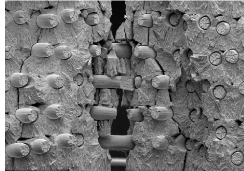
Figure 2: Cross-section of W f /W composite after a Charpy impact test: The tungsten fibres show ductile deformation and pull-out leading to increased toughness of the composite [7].
