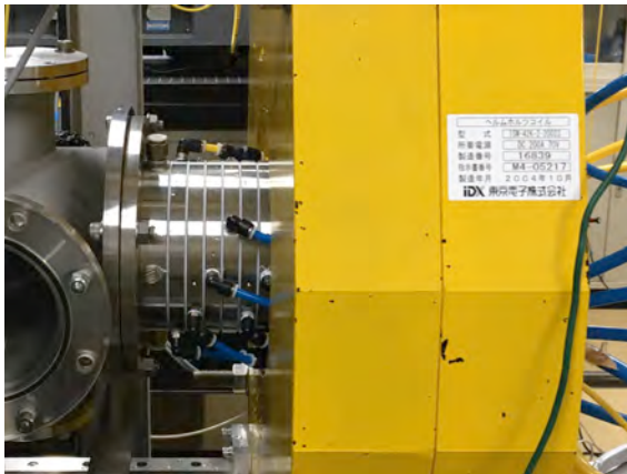
Figure 2. Schematic of the cascade arc discharge apparatus developed.
