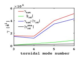
Figure 1. Growth radiative damping rates of RSAE vs toroidal mode number.
