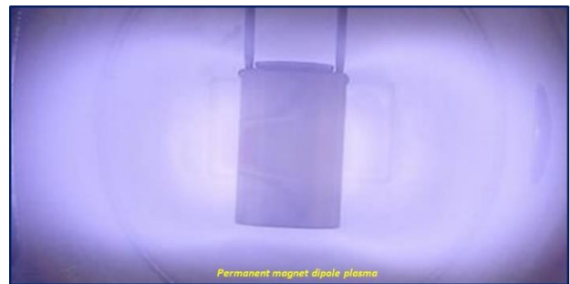
Fig. 2. Digital picture of the steady state permanent magnet dipole plasma. Note the alternate bright and dark regions, like the radiation belts of the Earth.
