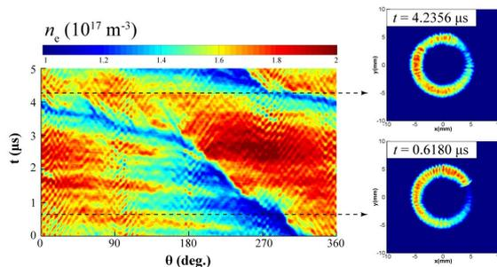
Fig. 2. Time evolution of the electron density in the high-density region on the  $\theta$ -axis together with typical electron density distributions at the  $x$ - $y$  plane. The  $\theta$ -axis is drawn at  $r = 5.0$  mm and  $z = 2.2$  mm. Figure is reproduced from Ref. [7].
