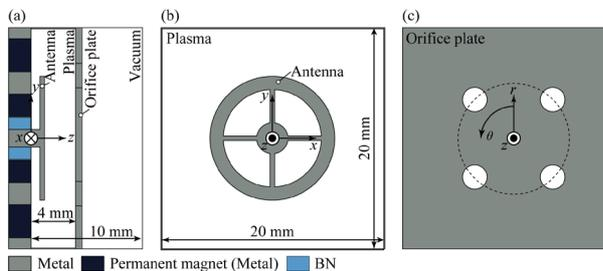
Fig. 1. Schematic of the calculation model: (a) the  $z$ - $x/y$  plane, (b)  $x$ - $y$  plane at the antenna, and (c)  $x$ - $y$  plane at the orifice plate. Figure is reproduced from Ref. [7].
