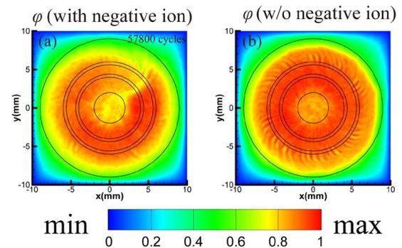
Fig. 3. Distributions of (a) the normalized potential on the  $x$ - $y$  plane with negative ions and (b) without negative ions. Figure is reproduced from Ref. [6].
