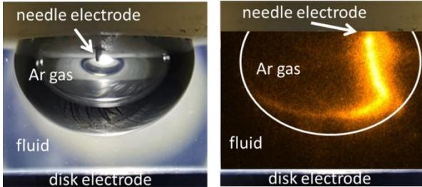
Figure 1 Ar bubble prior to the discharge and during the discharge. The discharge with +5kV between the needle and disk electrodes was imaged with a fast ICCD, 15 ns exposure, 360 ns after the start of the discharge.
