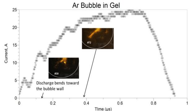
Figure 2 Discharge propagation in Ar bubbles in gel recorded with PI MAX ICCD with gate width (exposure) of 5 ns and a 5 ns step for the first 100 shots and longer thereafter. A typical current trace is shown as a reference.
