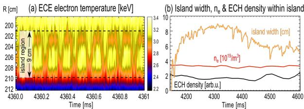
Fig.1. (a)  $T_e$  contour, (b)  $W$ ,  $n_e$  and ECH power density.
