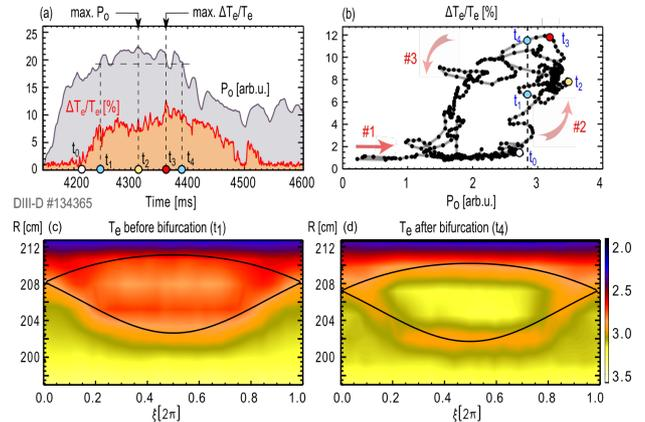
Fig. 2.  $P_o(t)$  and  $\Delta T_e(t)/T_e(t)$ , (b)  $P_o(t)$  vs  $\Delta T_e(t)/T_e(t)$ , (c/d)  $\Delta T_e$  before/after bifurcation at the same  $P_o$ .
