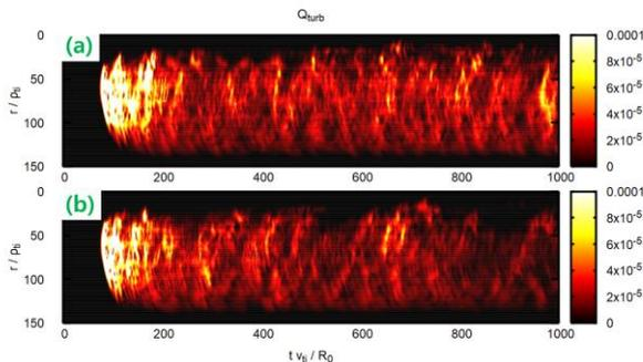
Fig. 1. Time evolution of the radial turbulent heat flux (a) at 2 MW input power and (b) at 0.5 MW input power.
