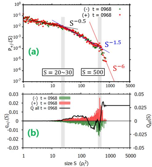
Fig. 3. Size PDF of heat flux eddies (a) and total heat flux contribution by eddy size (b) at burst phase.
