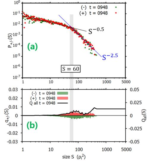
Fig. 2. Size PDF of heat flux eddies (a) and total heat flux contribution by eddy size (b) at quiescent phase.
