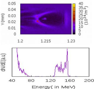
and the corresponding electron energy spectrum. The injected bunch becomes monoenergetic in the case of the asymmetric laser pulse because the pulse of the front part of the laser pulse becomes shorter. When the pulse gets compressed and becomes asymmetric, the emittance of the electron bunch reduces. Hence, the pulse asymmetry can be considered as one of the controlling knobs for the emittance of the accelerated bunch.
