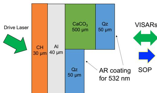
Fig. 1 Schematic setup in laser shock experiments.
