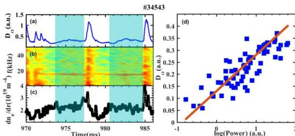
Fig. 1. (a)  $D_\alpha$  signal in the lower divertor, (b) the frequency spectrum of the  $J_{sat}$  on the divertor target, (c) the density gradient in the pedestal, (d) the amplitude of the  $D_\alpha$  versus the power logarithm of the CP on the divertor target plate.
