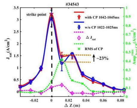
Fig. 2. The effect of the CP on the distribution of the particle flux: Left Y-axis: The profiles of saturate ion current density  $J_{sat}$  on the divertor target with and without CP; Right Y-axis: the RMS of  $J_{sat,CP}$  on the outer divertor target and the increment of the  $J_{sat}$ .
