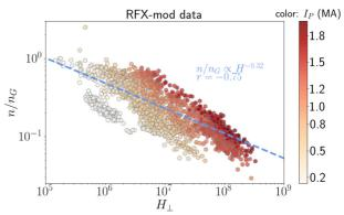
1. In RFX-mod a clear relation between the first-principle MHD dimensionless Hartmann number H (here computed using the perpendicular Braginskij plasma viscosity) and the Greenwald density  $n_G$  is found.
