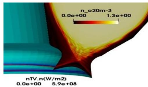
Fig.1. Density and divertor heat flux during natural 4MJ ELM crash in ITER 15MA/5.3T scenario.
