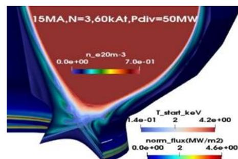
Fig.2. Density, Poincare plot and divertor heat flux in ELM suppressed stage by RMPs N=3, 60kAt in ITER.
