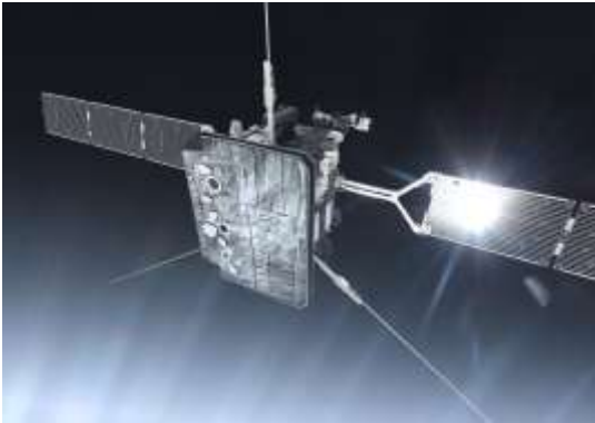
Figure 1. Artist's impression of the front view of the Solar Orbiter spacecraft, showing the heat shield with the open apertures for the remote sensing instrument
