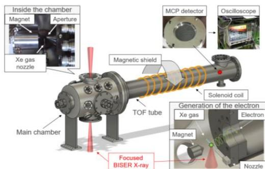
FIG. 1. Schematic diagram of the magnetic bottle electron spectrometer.
