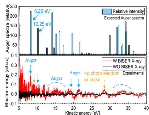
FIG. 2. (a) A relative Auger electron intensity. (b) Electron spectra generated in BISER and Xe interaction.
