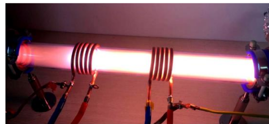
Fig. 1 Typical discharges driven by single (one-leg) and dual (two-leg) antennas.
