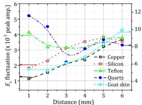
Fig.2 Variation of peak amplitude of fluctuating frequencies in electric field ( $E_z$ ) with axial distance of plasma jet
