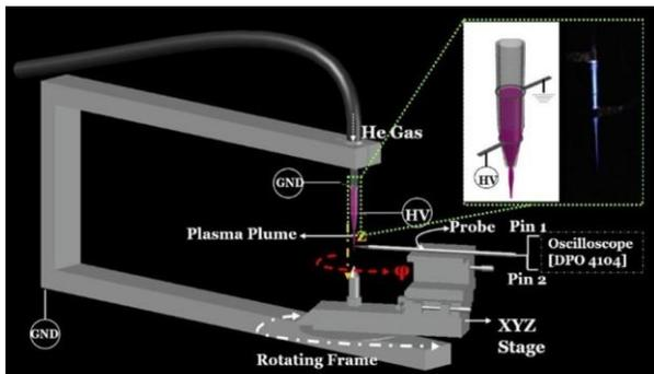
Fig. 1. Schematic diagram of experimental set-up of plasma jet with rotating frame designed to measure the electric field in axial and poloidal direction of jet
