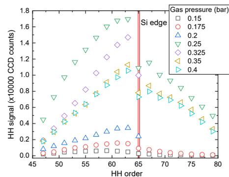
FIG.2 HH signal observed under various valve gas pressures.
