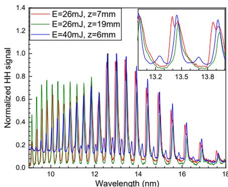
FIG.1 HH spectra for two focusing conditions. Laser pulse energies on target were 26 mJ or 40 mJ.
