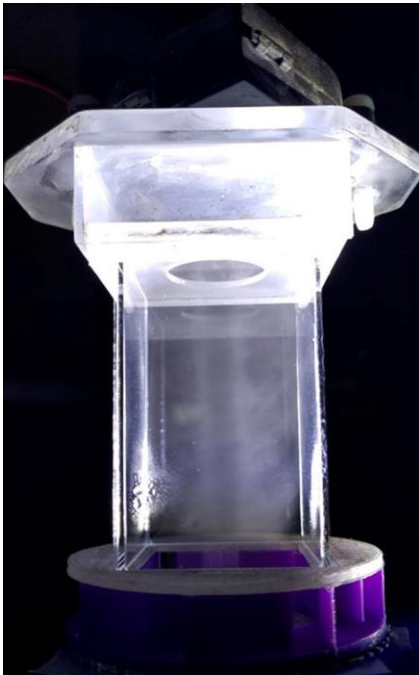
Figure 1. The spiral vortex inside the cell is visualized by the water mist. Exhaust fan, buffer tank, square cell, and flow vanes are sequentially shown from the top to the bottom (left). A 10-cm filamentary discharge is produced at 29 kVpp (right).
