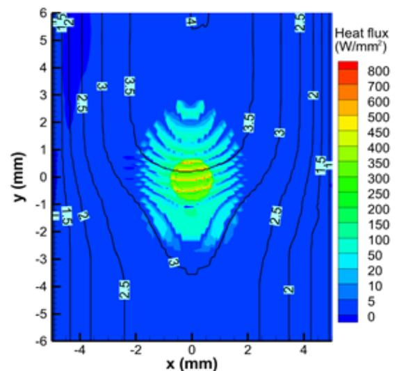
**Figure 1:** Calculated distribution of the heat flux to the workpiece surface during deposition of the fourth layer for the parameters of Zhao et al. [3]. The contour lines indicate the build height above the original substrate surface in mm. The arc is moving in the  $-y$  direction.
