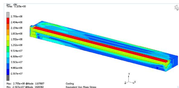
**Figure 2:** Von Mises stress distributions predicted by the coupled MHD-FEA model after deposition of the first layer. The scale is from 0 to 270 MPa in 27 MPa increments. The substrate is 51 mm long  $\times$  21 mm half-width  $\times$  6 mm thick.
