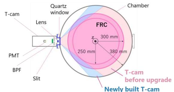
**Figure 2.** Comparison of the field of view, newly built T-cam and before upgrade.
