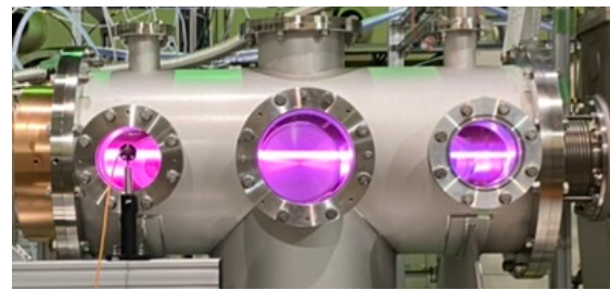
Figure 3. First hydrogen plasma viewed from the observation port of the differential pumping chamber (discharge current 20A).
