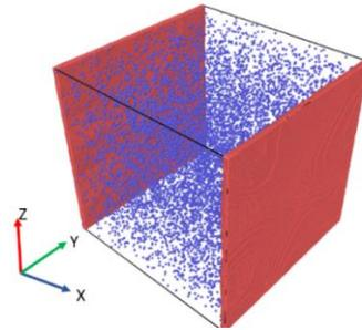
Fig. 1 Snapshot of the confined simulation system. Brown colour shows the walls and blue dots show He atoms.
