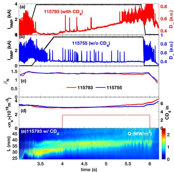
Figure 1. The effective heat flux reduction by  $\text{CD}_4$  injection in EAST #115793 discharge and the comparison with another discharge #115755 without any impurity injection. (a)(b)
