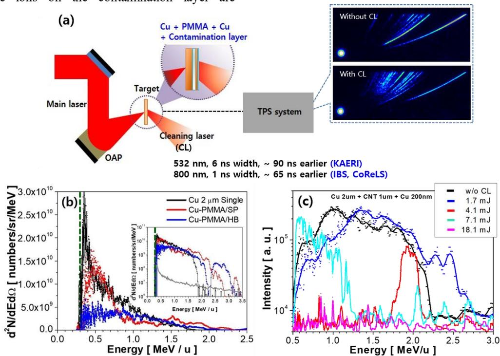
**Figure 1.** (a) Experimental schematics for ILEF target with cleaning laser to reduce the effect of ES field by contamination layer. (b) Non-thermal energy spectra of C<sup>6+</sup> ions obtained from IEDL targets. (c) Non-thermal energy spectra of C<sup>6+</sup> ions obtained from ILEF target with variable cleaning laser.
