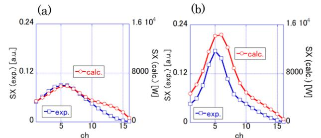
Figure 1 Comparison of soft X-ray intensity distribution (a) in small  $V_t$  and small W accumulation and (b) in large  $V_t$  and large W accumulation.
