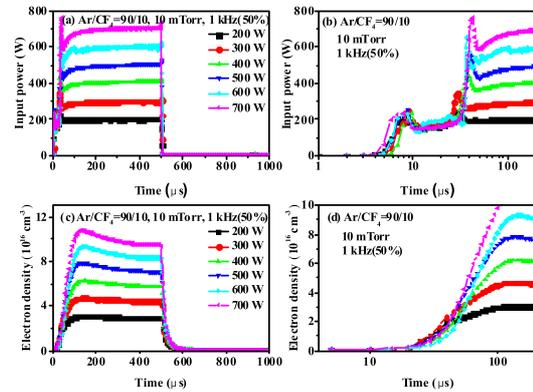
FIG. 2. Temporal evolutions of the input power and the electron density for different powers at 10 mTorr in Ar/CF<sub>4</sub> discharges, with a pulse frequency of 1 kHz and 50% duty cycle, (a) the input power for the whole pulse period, (b) the input power until 200  $\mu$ s in the initial pulse stage, (c) the electron density for the whole pulse period, and (d) the electron density until 200  $\mu$ s in the initial pulse stage.
