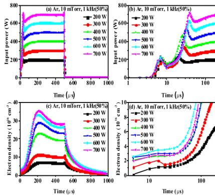
FIG. 1. Temporal evolutions of the input power and the electron density for different powers at 10 mTorr in Ar discharges, with a pulse frequency of 1 kHz and 50% duty cycle, (a) the input power for the whole pulse period, (b) the input power until 200  $\mu$ s in the initial pulse stage, (c) the electron density for the whole pulse period, and (d) the electron density until 200  $\mu$ s in the initial pulse stage.
