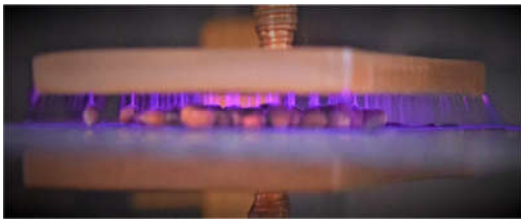
Fig1. Photograph of NTP during the treatment of seed.
